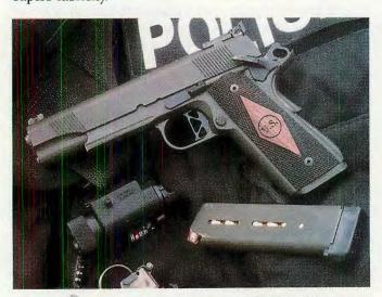
The tactic light can be removed from the RECON RAIL in about two seconds. Its Wilson magazine held eight rounds of .45 ACP.
